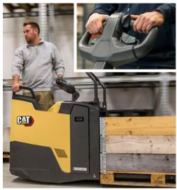
Models are available with foldable or fixed platforms, 2.0 or 2.5 tonne load capacities and a choice of three chassis lengths. They can also be equipped for Li-ion or lead-acid battery use. NPV20N3 and NPV25N3 folding platform versions feature fold-up/fold-down protective side bars.
